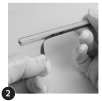
Remove backing from adhesive tape.
